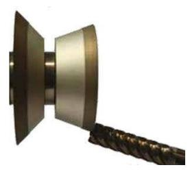
Clearance angles grinding on the cutting edge of a tool reduces the contact area between the tool and the workpiece during drilling or milling processes. One or two clearance angles are usually ground on the face. Up to two clearance angles / clearances can be produced on the circumference; on some tools these take the form of radial clearance grinding. For grinding clearance angles 11V9 cup wheels or similar geometries are typically used.
