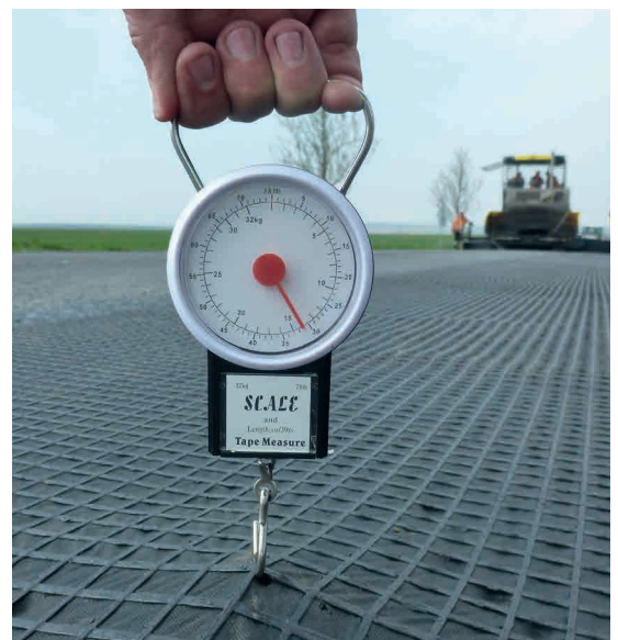
Pic. 8: Adhesion pull out test
